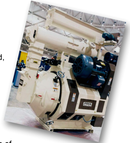
Large electric motors are used to power pellet mills, which compact wood particles and extrude them as pellets through small openings in steel dies.
