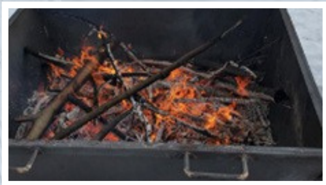
Kiln with a bed of coals and ready for feedstock additions.
