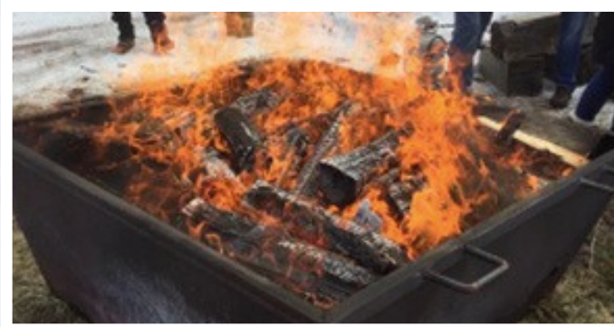
Biochar kiln with a good flame cap.
